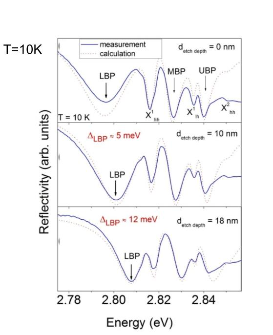
Spectral shift of the Bragg polaritons with change of the top layer thickness
