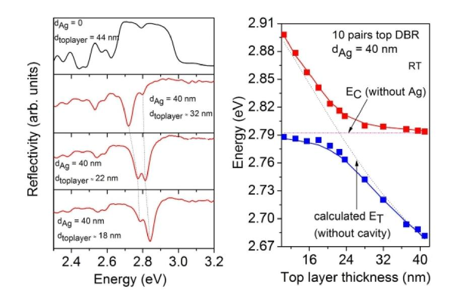
Reflectivity of sample without and with Ag layer for different top layer thicknesses
