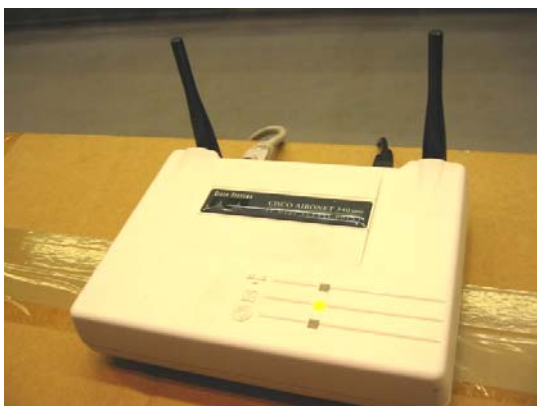
Foto 6: Accesspoint Cisco AIRONET 340 Series (IEEE 802.11b)
